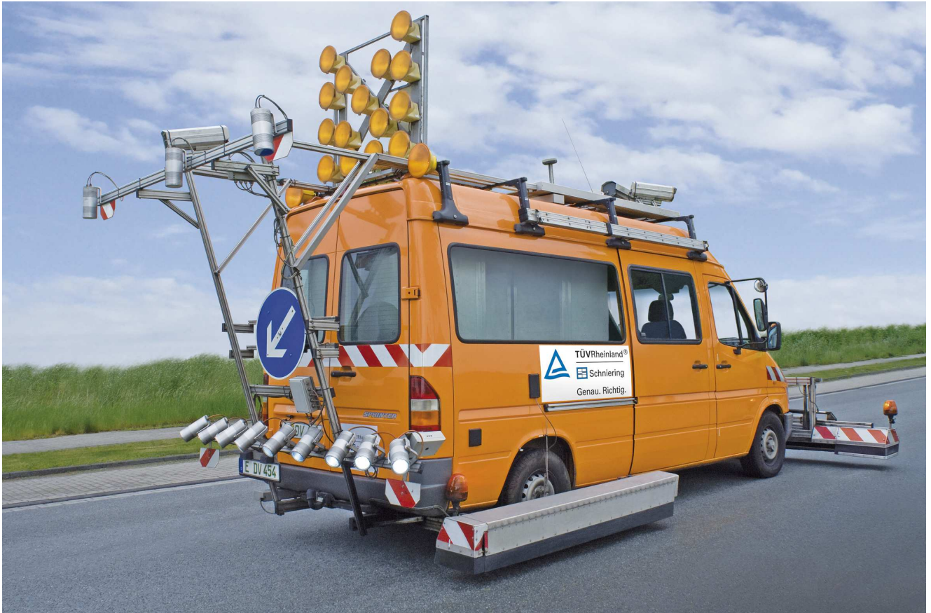
Multi-functional Survey System ARGUS® with Macro Video Recording and nine High-Performance Stroboscopes
